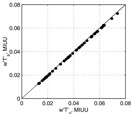
**Figure 13.** Thirty-minute means of  $\overline{w'T'_s}$  plotted against  $\overline{w'T'_v}$ , both derived from measurements at Östergarnsholm with the MIUU-instrument at 10 m during October, 1999 and computed with (A1) and (A2), respectively.
