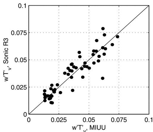
**Figure 14.**  $\overline{w'T'_v}$ , measured with the R3 sonic and corrected for the crosswind effect according to Kaimal and Gaynor [1991] plotted against the same quantity derived from simultaneous measurements with the MIUU-instrument and obtained with (A2). Same data set as in Figure 13.
