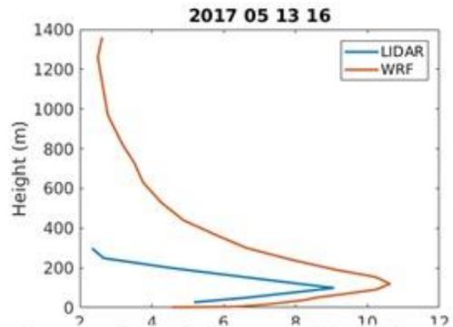
A comparison between LIDAR and tower measurements at Östergarnsholm during a low-level jet event the 13th of May 2017. Figure made by: Nina Svensson
